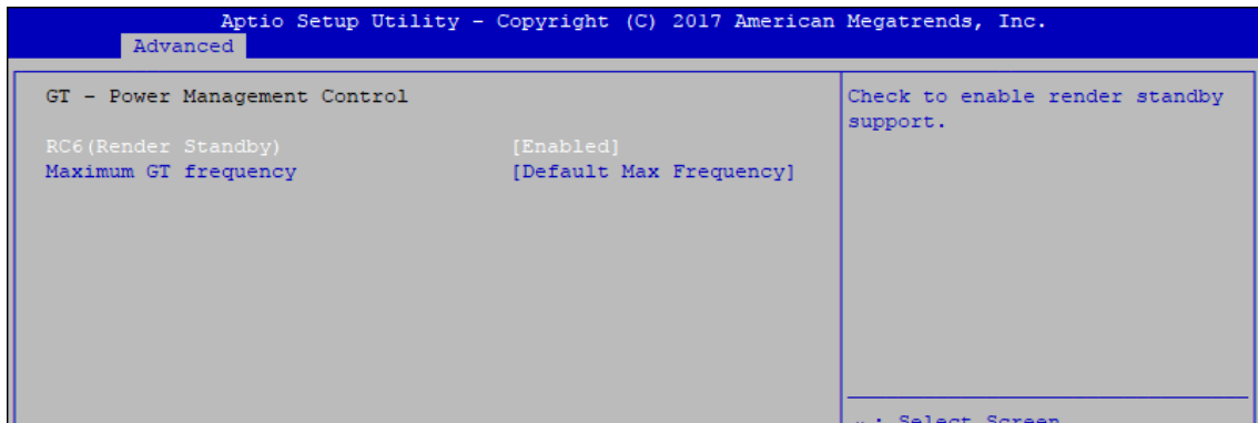
Figure 4-3-2-2: GT – Power Management Control
