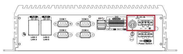
This system supports 6V to 36V DC power input by terminal block in the rear side. In normal power operation, power LED lightens in solid green. Supports up to 80V surge protection.
