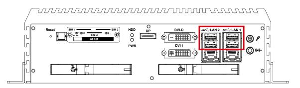
There are 4 USB 3.0 connections available supporting up to 5GB per second data rate in the front side of Echo-236F. It also compliant with the requirements of Super Speed (SS), high speed (HS), full speed (FS) and low speed (LS).
