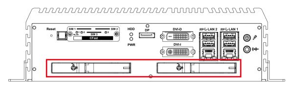
There are 2 front-access 2.5" SSD/ HDD trays in the front side of Echo-236F. Just trigger to open the SSD/ HDD tray, up to 4TB is available.
