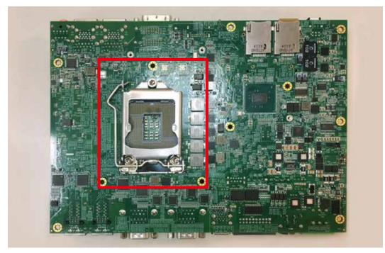
Step 4 Open CPU slot. (Be careful CPU pin)
