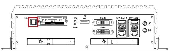
The Power Button is a non-latched switch with dual color LED indication. It indicates power status: S0, S3 and S5. More detail LED indications are listed as follows:
