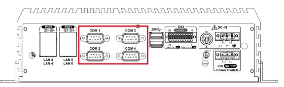
Serial port 1 to 4 (COM 1 to 4) can be configured for RS-232, RS-422, or RS-485 with auto flow control communication. The default definition of COM 1 and COM 2 is RS-232, if you want to change to RS-422 or RS-485, you can find the setting in BIOS.
