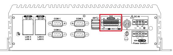
There is a 16-bit (8-bit DI, 8-bit DO) connectors in the rear side. DI/DIO support NPN(sink) and PNP(Source) mode, Each DI channel is equipped with a photocouper for isolated protection. Each DO with isolator chip, Config by a Jumper for each DIO connector. DO Safety-Related Certifications:
