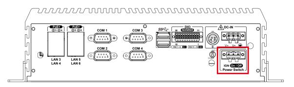
It is a 2-pin power-on or power-off switch through Phoenix Contact terminal block. You could turn on or off the system power by using this contact. This terminal block supports dual function of soft power-on/ power-off (instant off or delay 4 second), and suspend mode.
