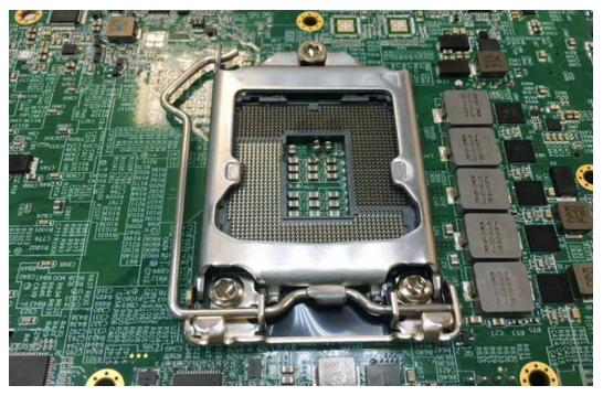
**Step 5** Installing CPU on the slot.
