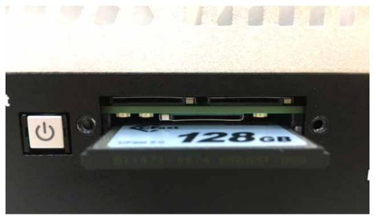
Step 4 Insert CFast card and push to lock.
