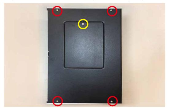
**Step 3** Remove bottom four F#6-32(red) and one F-M3(yellow) screws.
