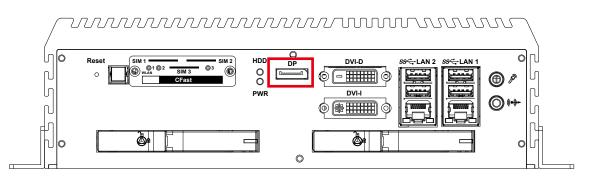
Onboard Display Port support auxiliary channel dual mode, connection supports up to 4096x2304 resolution at 60 Hz.
