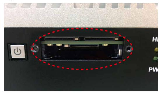
**Step 3** Before Inserting CFast & SIM Card, make sure the system power is not plugged.
