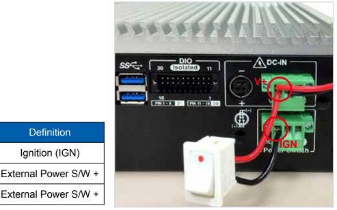
For testing purpose, you can refer to the picture above to simulate ignition signal input controlled by a latching switch.
