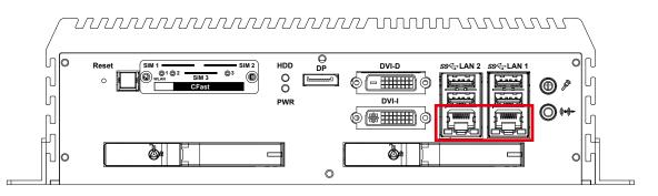
There are 2 8-pin RJ-45 jacks supporting 10/100/1000 Mbps Ethernet connections in the front side. LAN 1 is powered by Intel i219 Ethernet Phy; LAN 2 is powered by Intel I210 Ethernet engine. When both LAN 1 and LAN 2 work in normal status, iAMT 11.0 function is enabled.
