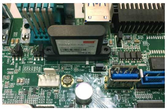
Step 4 Lock two M2 screws with slot.
