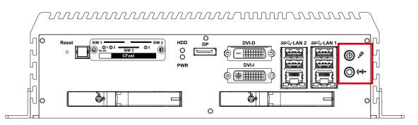
There are 2 audio connectors, Mic-in and Line-out, in the front side of Echo-236F. Onboard Realtek ALC892 audio codec supports 5.1 channel HD audio and fully complies with Intel<sup>®</sup> High Definition Audio (Azalia) specifications. To utilize the audio function in Windows platform, you need to install corresponding drivers for both Intel CM236 chipset and Realtek ALC892 codec.
