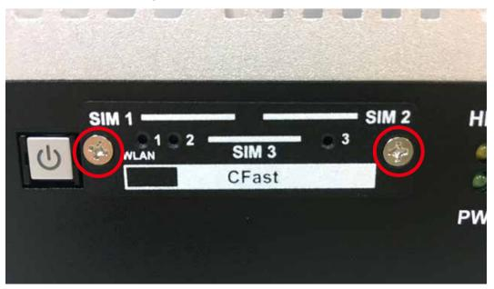
Step 2 Remove CFast Card and SIM Card cover.
