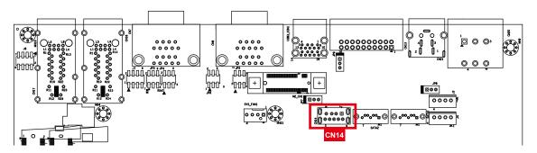
The USB 3.0 connections available supporting up to 5GB per second data rate. It also compliant with the requirements of SuperSpeed (SS), high speed (HS), full speed (FS) and low speed (LS). The pin assignments of CN14 are listed in the following table:
