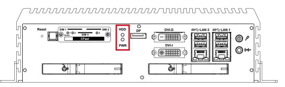
HDD LED/ Yellow: A Hard Disk/ CFast LED. If the LED is on, it indicates that the system's storage is functional. If it is off, it indicates that the system's storage is not functional. If it is flashing, it indicates data access activities.
