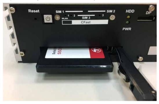
**Step 3** Installing 2.5" SSD/HDD into the tray.
