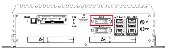
The DVI-D connector on the front panel supports DVI display. This connector can either output DVI signal. The DVI output mode supports up to 1920 x 1200 resolution and output mode supports up to 1920 x 1200 resolution. The DVI is automatically selected according to the display device connected. You will need a DVI-D cable when connecting to a display device.
