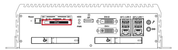
There is a CFast socket on the front panel supporting Type-I/II Compact Flash card. It is implemented by a SATA III Port from CM236 PCH. Be sure to disconnect the power source and unscrew the CFast socket cover before installing a CFast card. The Echo-236F does not support the CFast hot swap and PnP (Plug and Play) functions. It is necessary to remove power source first before inserting or removing the CFast card.
