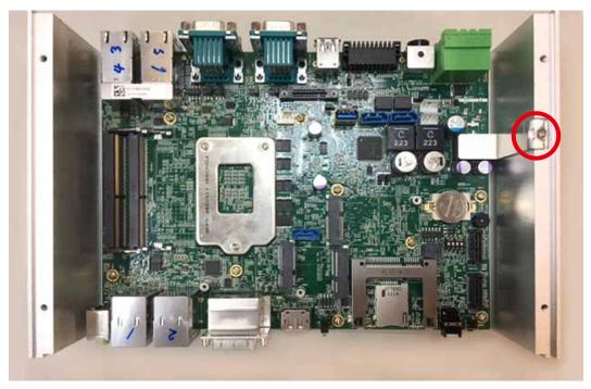
**Step 2** Remove eleven PH-M3 screws and pick up mother board.
