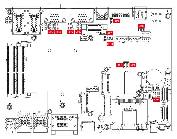
The figure below is the top view of the system board, and it shows the location of the jumpers and the switches.
