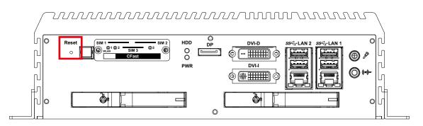
It is a hardware reset switch. Use this switch to reset the system without power off the system. Press the Reset Switch for a few seconds, then reset will be enabled.
