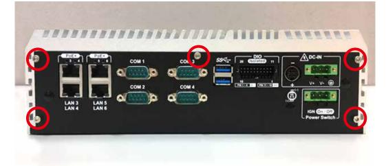
**Step 3** Remove bottom four F#6-32 screws.
